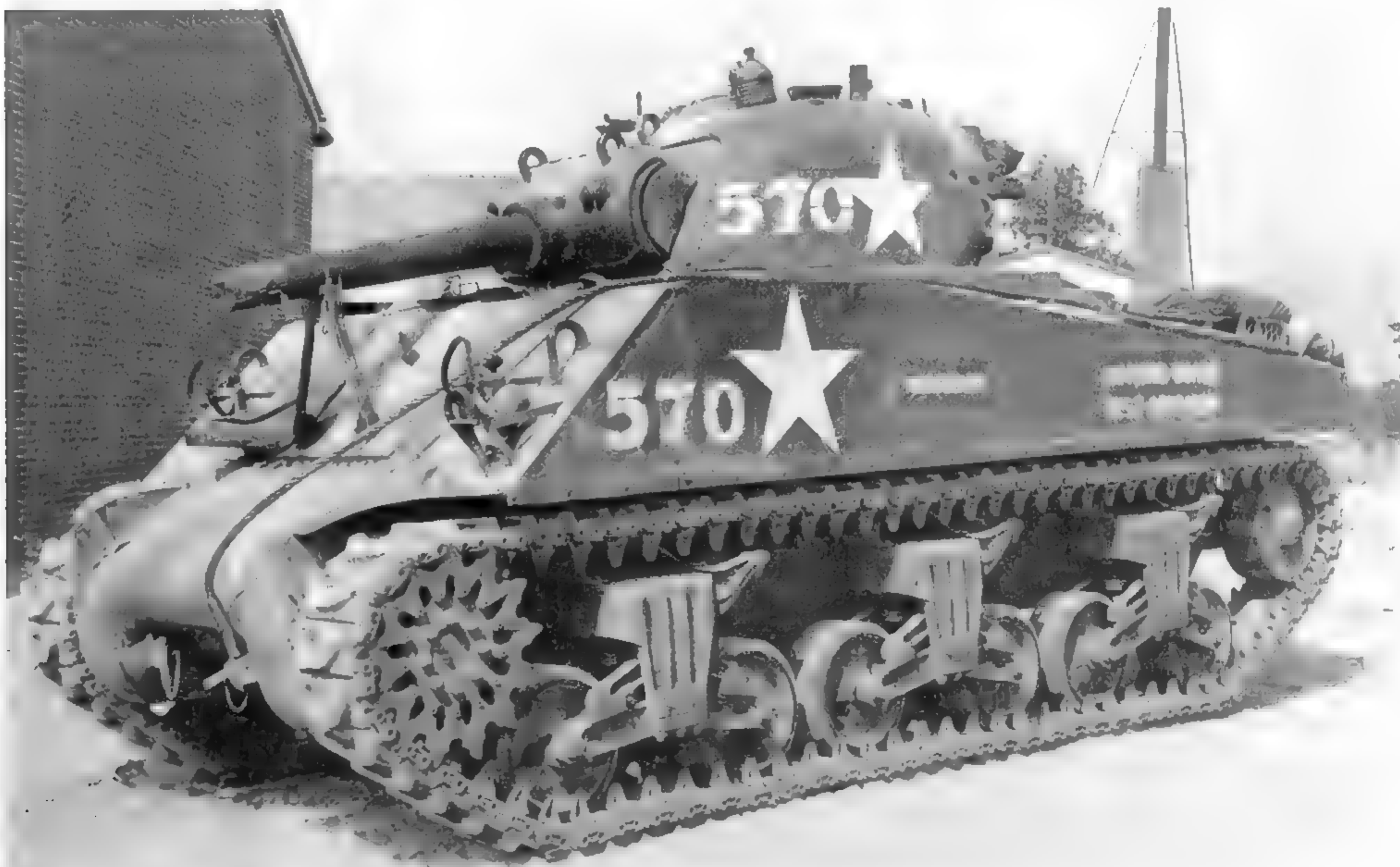
A 105mm howitzer-armed M4 undergoes tests by the Armor Board at Ft. Knox. It has the old style vertical volute suspension, as used on the M3 Lee. (Photo courtesy of the Patton Museum)
